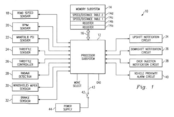
Figure 1 is a block diagram of the '781 system. Ex. 1001, 5:42–44. System 10 includes processor subsystem 12 ("for example, a microprocessor"), and memory subsystem 14 connected by bus 16 to processor subsystem 12. *Id.* at 5:54–58. State sensors and level sensors, including road speed sensor 18, rpm sensor 20, manifold pressure sensor 22, throttle sensor 24, windshield wiper sensor 30, and brake sensor 32, collectively monitor the operation of
