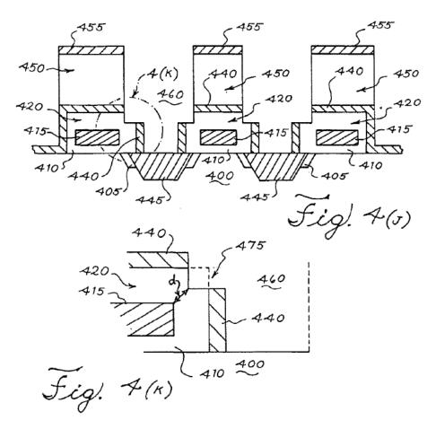
Figures 4(J) and 4(K) illustrate the structure of the semiconductor device of the '552 patent after the second etch for removing the etch stop layer from the contact regions 460 and 465 is completed. As shown in Figures 4(J) and
