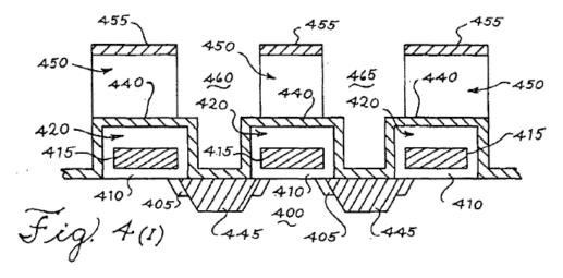
Figure 4(I) illustrates additional structures deposited and etched over the structure described in Figure 4(D), such as second dielectric layer 440 (called etch stop layer), blanket layer 450, and photoresist mask layer 455. *Id.* at col. 9, ll. 33–39; col. 11, ll. 63–65; col. 12, ll. 34–42. According to the '552 patent, etch stop layer 440, e.g., silicon nitride layer 440, depicted in Figure 4(I) is distinct or different from the underlying TEOS insulating
