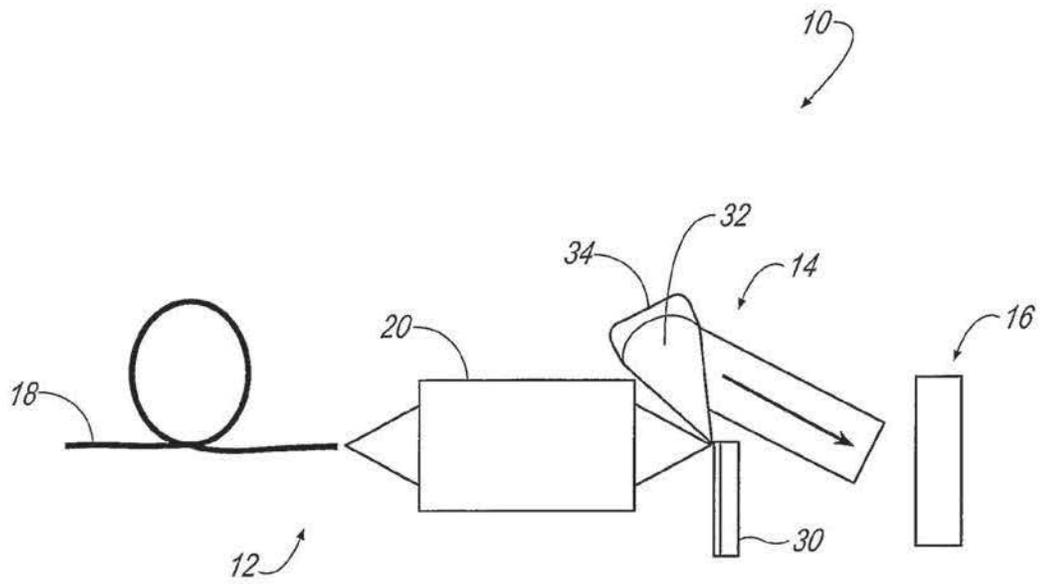
(57) Abstract: A method and apparatus is disclosed for performing lithography operation. A fiber laser (18) is provided that generates laser light that is used by adaptive optics (20) to focus the laser light onto a plasma target (30) to generate plasma as a source of EUV radiation.
