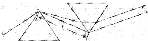
Figure 11.26 Prisms are the most common way of introducing GVD compensation. A prism geometry can be arranged so that the blue components transverse the prism path in a shorter length of time than the red components.
