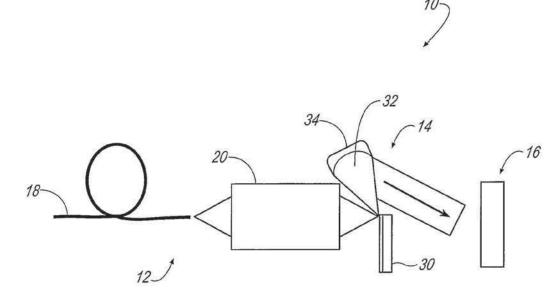
(57) Abstract: A method and apparatus is disclosed for performing lithography operation. A fiber laser (18) is provided that generates laser light that is used by adaptive optics (20) to focus the laser light onto a plasma target (30) to generate plasma as a source
