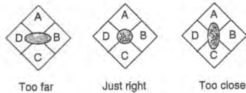
Figure 12.51 The separation between the laser and the compact disk is critical for the correct operation of the CD player. A clever astigmatic autofocus mechanism is used to maintain this distance.
