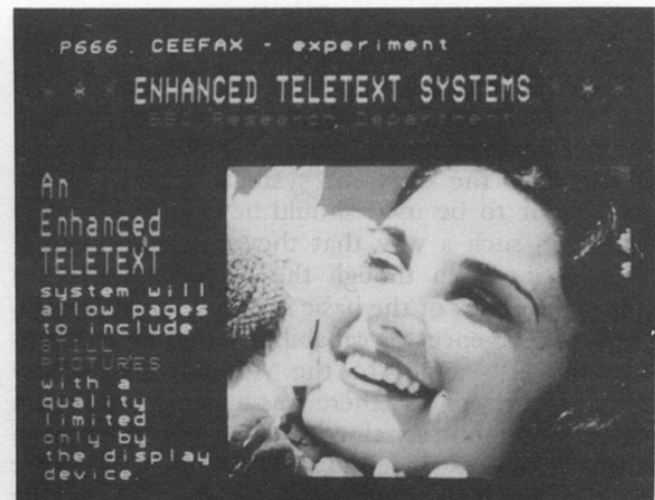
Fig. 7 - An RGB television picture inset in a teletext page
