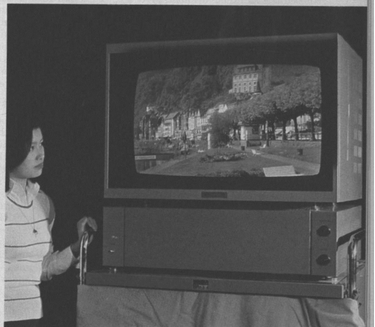
Wide-screen high-resolution monitor developed by NHK and Matsushita has 30-inch-diagonal screen, 5:3 aspect ratio. Phosphor dots are much smaller than on conventional shadow-mask tubes, and NHK uses a digital beam-convergence system.
