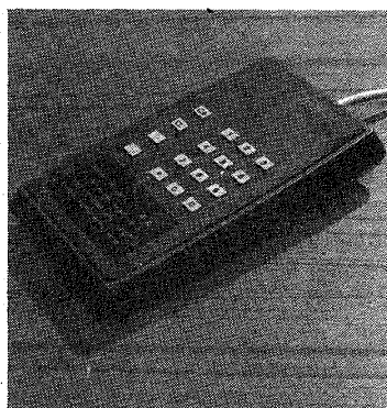
▲ Fig. 3. Basic keypad used in a Viewdata terminal, providing ten numerals and a few other keys.
