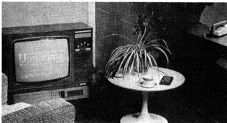
▲ Fig. 2. Home terminal for Viewdata, with television set, telephone (right) and keypad on the table.
