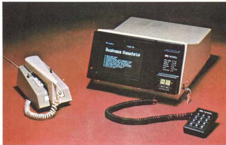
Figure 8.2. Typical business TV terminal.
