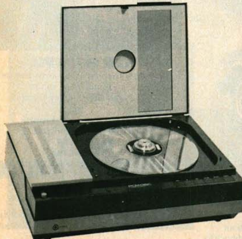
Optical disc-player system made by Mitsubishi and others has a dynamic range exceeding 98 dB. Spiral tracks of pits on discs (magnified at right) are about 0.6 microns wide, have a protective plastic coating against dust and smears.
