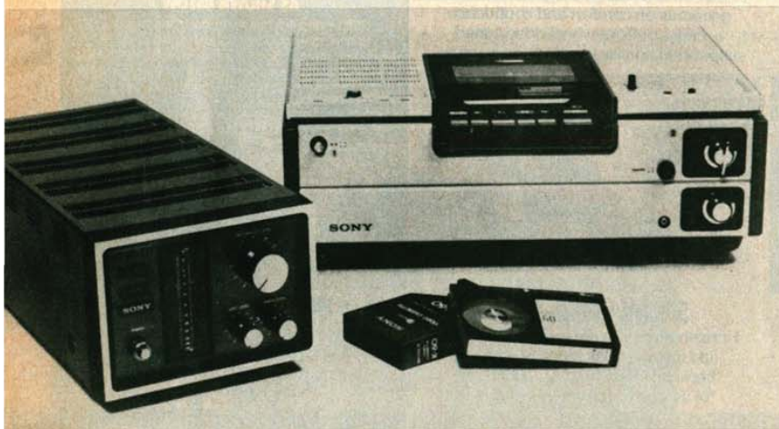
Recording/playback adapter (left) for Sony's or other video-cassette recorders puts digitized audio signals on the cas-
