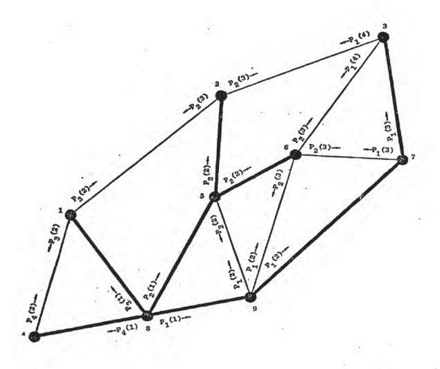
Figure 3.4. SUBOPTIMAL REVERSE PATH FORWARDING INITIATED FROM NODE 8.
