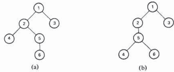
Fig. 3. (a) Shortest path tree for network of Fig. 2(a) after the length of the line 2 → 4 increase to 6. (b) Modified tree after the length of line → 5 decrease to 2.
