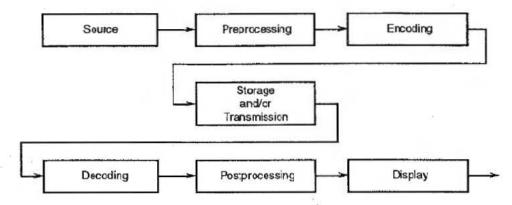
Figure D.1 -- Coding and decoding process
