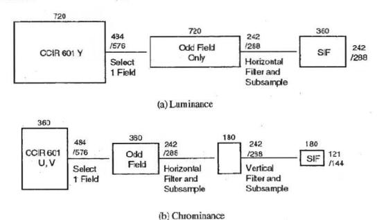
Figure D.12 -- Conversion from CCIR 601 into SIF
