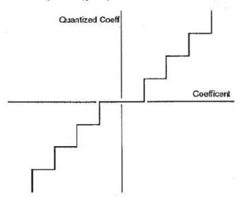
Figure D.35 -- Dead zone quantizer characteristic
