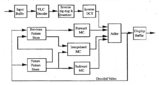
Figure D.7 - Simplified decoder block diagram
