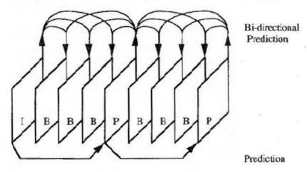
Figure 1 -- Example of temporal picture structure
