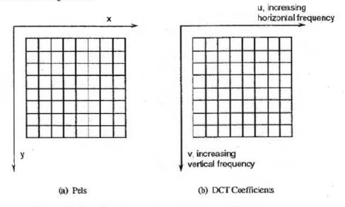
Figure D.28 -- Transformation of pels to coefficients
