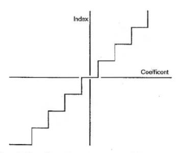
Figure D.29. -- Uniform quantizer characteristics
