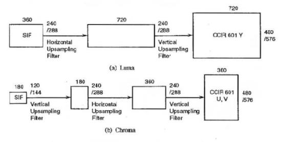
Figure D.41 -- Simplified decoder block diagram
