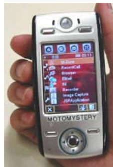
Personal Server prototype integrated into a Motorola E680 ® Intel ® XScale ™ /Linux-based cell
