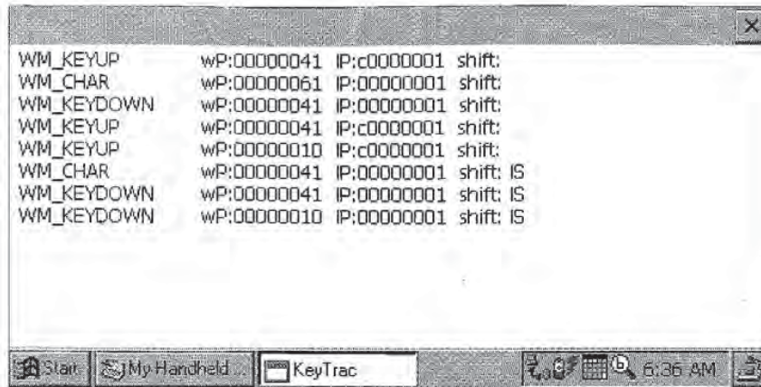
Figure 3-4. The KeyTrac window after a Shift-A key combination followed by a lowercase a key press.
