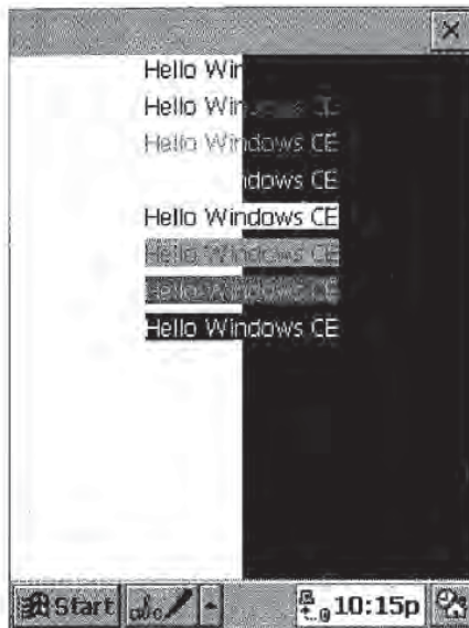
Figure 2-2. TextDemo shows how the text color, background color, and background mode relate.
