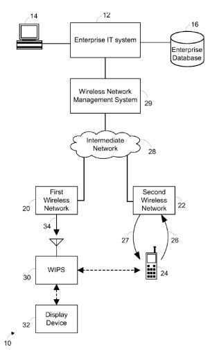
Figure 1 depicts wireless communication system 10 having enterprise information technology (IT) system 12 connected to one or more personal computers 14 and centralized enterprise database 16. *Id.* at 3:62–4:6. Enterprise IT system 12 uses wireless network management system 29 to communicate with first wireless network 20 and second wireless network 22 via intermediate network 28, which may be a wide-area network (WAN) or a local-area network (LAN). *Id.* at 4:34–41.
