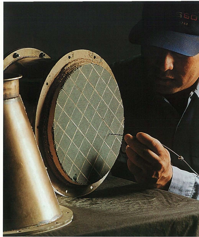
Diesel particulate filter cores made of specialty ceramics such as cordierite and silicon carbide (shown) are studied for particle collection efficiency, resistance to exhaust heat, buildup of backpressure, and completeness of regeneration (cleaning).
