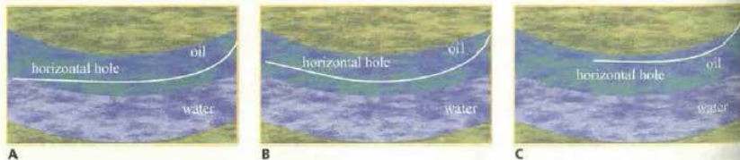
Fig. 4. Different hole layouts in a horizontal hole: A, undesirable orientation with respect to oil/water contact; B, hole tracking oil/water contact; C, the same as B, but with a shorter and better placed hole.
