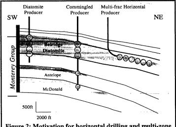
Figure 2: Motivation for horizontal drilling and multi-zone completions at the flanks of the Lost Hills Field.
