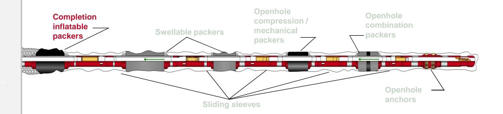
A packer that is inflated with fluid or cement to isolate zones in the open hole.
