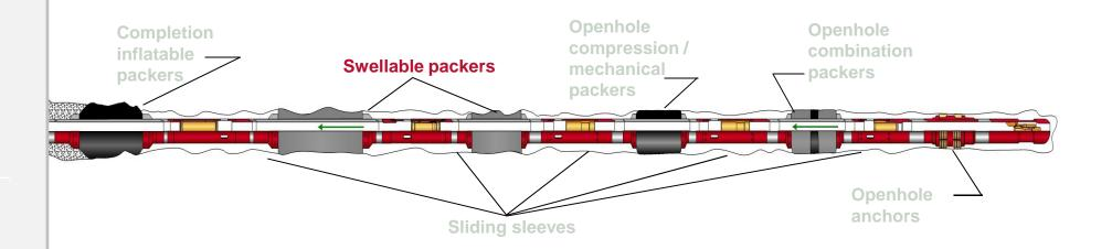
A packer that swells when it is in contact with well bore fluids. If no well fluids are present that we can carry our own expansion fluid.
