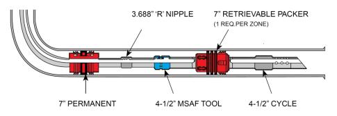
While Thomson's figure shows one ball-actuated sliding sleeve [blue] (which it called a "MSAF tool"), its text is clear that "[u]p to 9 MSAF tools [blue] can be
