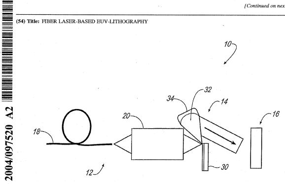
(57) Abstract: A method and apparatus is disclosed for performing lithography operation. A fiber laser (18) is provided that generates laser light that is used by adaptive optics (20) to focus the laser light onto a plasma target (30) to generate plasma as a source of EUV radiation.
