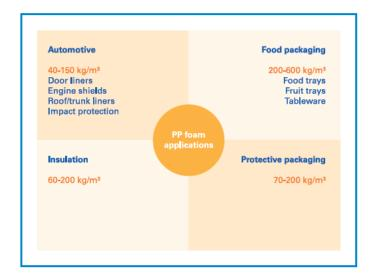
Figure 2: Some current applications for extruded PP foams
