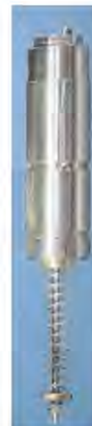
Fig. 2 Linear variable differential transformer (LVDT).
