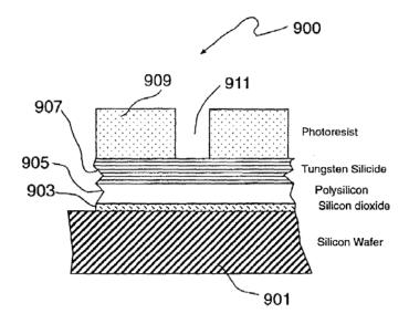
Figure 9 depicts substrate 901 having a stack of layers including oxide layer 903, polysilicon layer 905, tungsten silicide layer 907, and photoresist masking layer 909 with opening 911, from the treatment method shown in Figure 10, reproduced below. Ex. 1001, 17:58–18:57.
