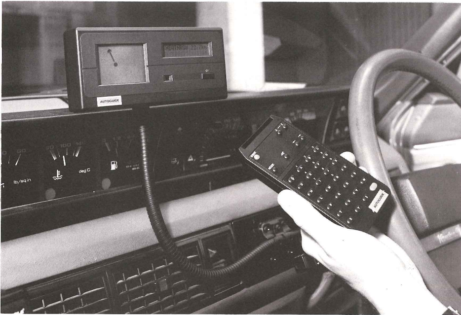
Fig. 43.3 The Autoguide screen (courtesy Department of Transport).
