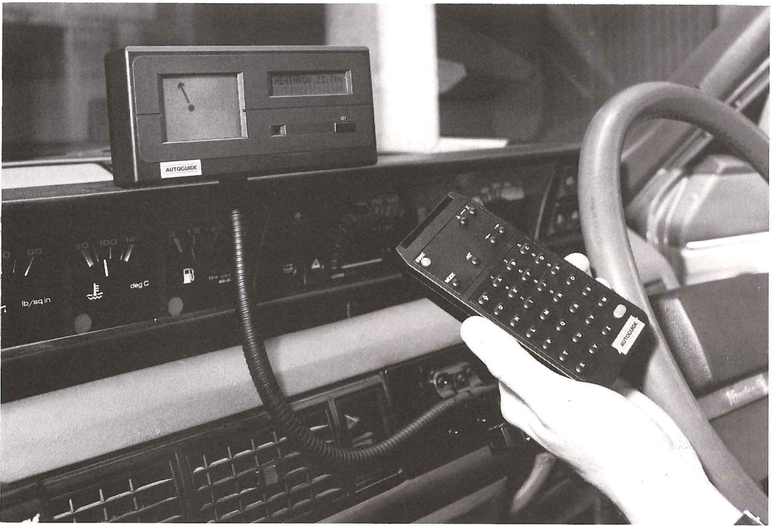
Fig. 43.3 The Autoguide screen (courtesy Department of Transport).
