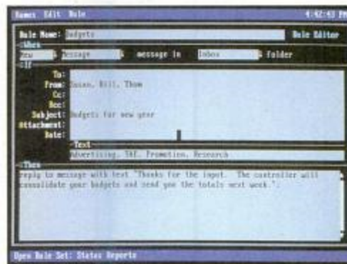
Using Beyond Mail rules, mail messages about a topic or from a certain person can generate other messages automatically.
