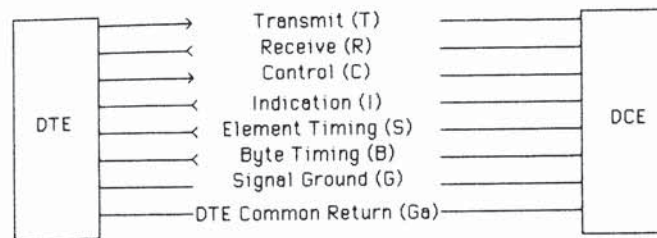
Figure 1.52 CCITT X.21 interchange circuits. Illustrates the X.21 interchange circuits by circuit type
