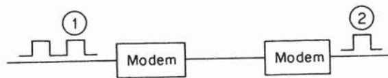
Figure 4.65 Internal modem delay time. Time difference from first bit transmitted (1) to first bit received (2) is denoted as total internal modem delay time ( 2D_m )
