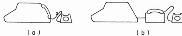
Figure 4.1 Varying coupler connections: (a) terminal with built-in coupler; (b) terminal connected to coupler
