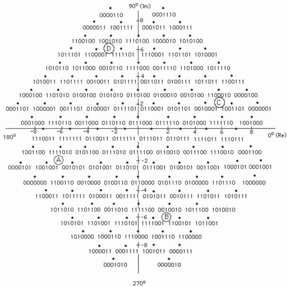
Figure 4.32 V.32 bis signal constellation and mapping for trellis-coded modulation at 14.4 kbps. A, B, C and D reference synchronizing signal elements
