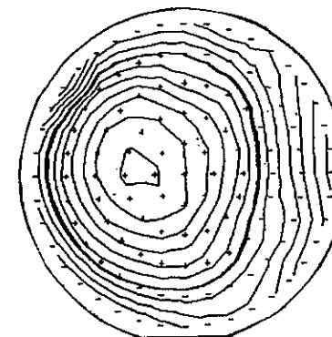
Fig. 15 Four-point probe contour map of a wafer after a furnace phosphorus predeposition.
