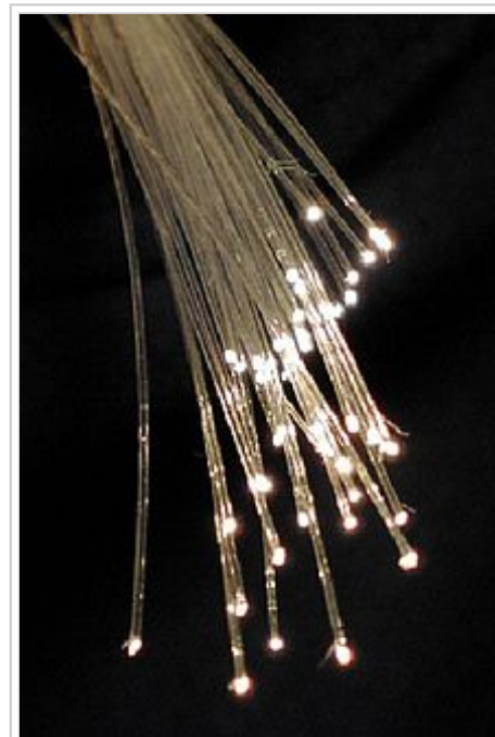
Bundle of optical fibers composed of high purity silica.
