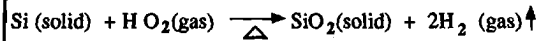
Figure 7.12 Reaction of silicon and water vapor to form silicon dioxide and hydrogen gas.
