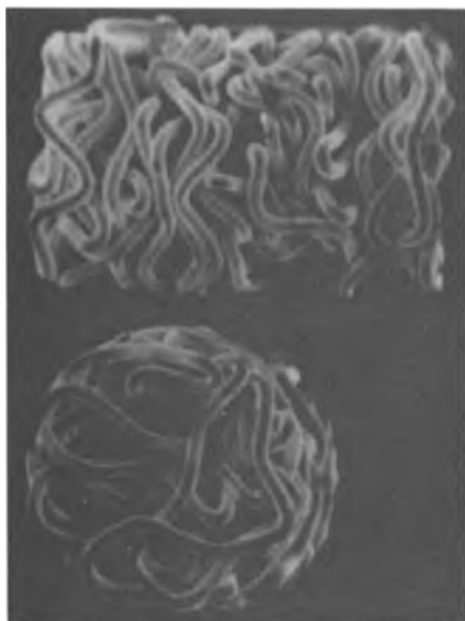
Figure 10-6 Button board connector showing connections to random wire configuration. (Courtesy of Cinch Connectors, a division of Labinal Components and Systems.)
