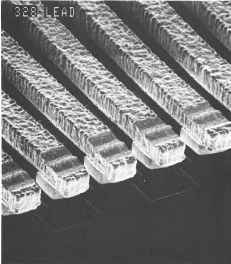
Figure 9-21 Single point thermosonically bonded TAB ILB 0.002" leads on 0.004" pitch. (Courtesy of Hughes Aircraft Company.)
