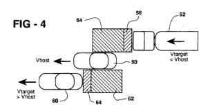
Figure 4 of the '927 patent illustrates radar coverage zones.
