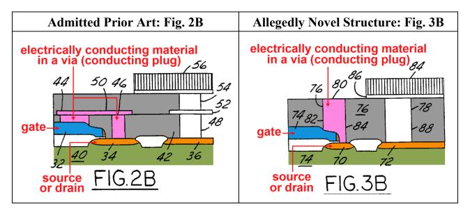
In both the admitted prior art (Figure 2B) and the allegedly novel structure of the '924 patent (Figure 3B), the gate is connected to a diffusion region (*i.e.*, a
