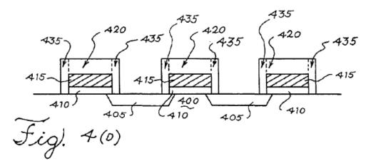
Figure 4(D) illustrates a cross-sectional view of a series of gates 415 (also called conducting layers or polysilicon layers) completely encapsulated in insulating material 420, e.g., TEOS (tetraethyl orthosilicate glass), where spacers 435 of the insulating material adjacent to the gates have substantially
