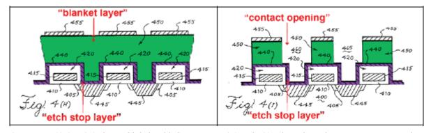
'552 Patent at 12:35-43 (color and labels added). Figures 4(H) and 4(I), where the etching process removes the blanket layer to create the contact openings, yet does not etch away the etch stop layer.
