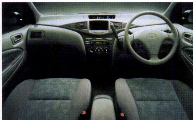
Instrumentation is digital, in the center top of the instrument panel, below which is a multipurpose display.
