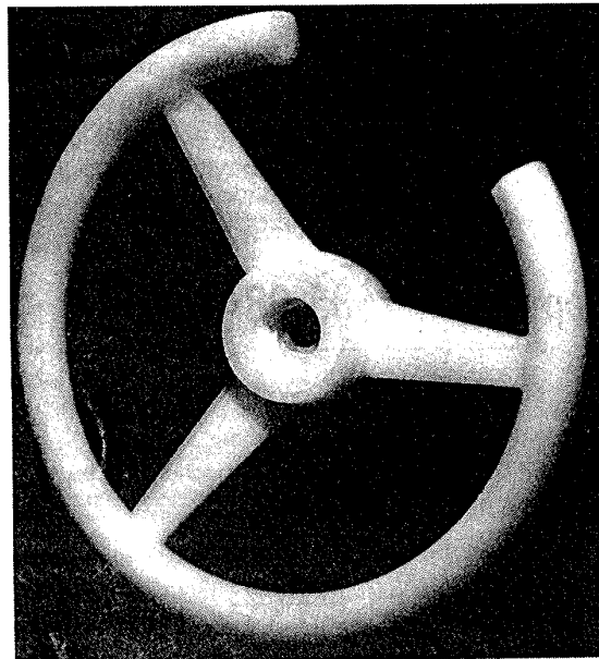
Figure 8.5 A steering wheel molded from a blend of 60% general purpose polypropylene and 40% foamable polypropylene (Tenite, Eastman Plastics). Molding conditions were: cycle time 35 seconds; melt temperature 193°C (380°F); mold temperature 4.4°C (40°F). [727]
