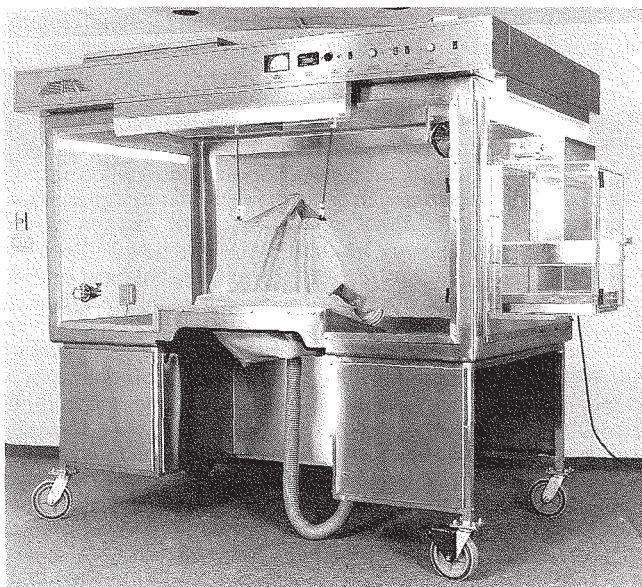
Fig 29. Stainless-steel half-suit isolator (courtesy, Laminar Flow).
