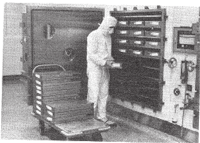
Fig 27. Aseptic loading of freeze-drier (courtesy, Upjohn).
