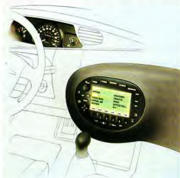
Visteon's Windows CE-based ICES multimedia system has information, communication, entertainment, safety, and security features.
