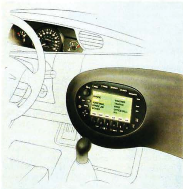
Visteon's Windows CE-based ICES multimedia system has information, communication, entertainment, safety, and security features.
