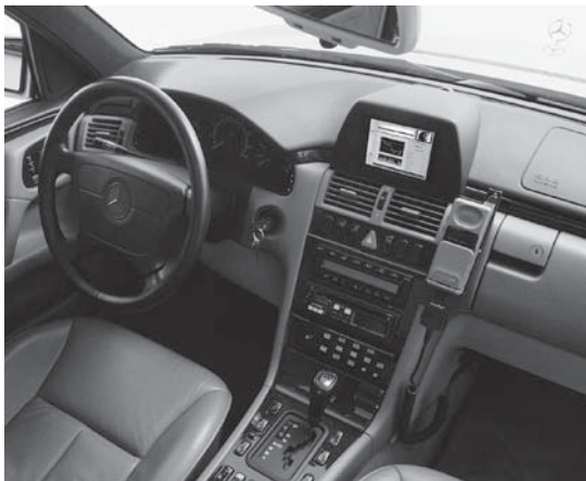
Figure 5. The front multimedia zone of the Internet car is accessible to both the driver and the navigator.
