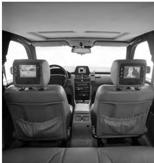
Figure 6. The rear passengers have access to multimedia units that contain screens, channel selectors for games, a computer, navigation tools, infrared transceivers, and audio outlets.
