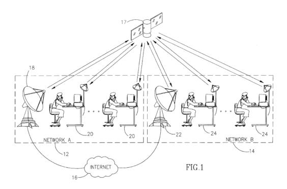
Figure 1 of the '073 patent depicts two satellite communication networks. *Id.* at 8:56–57. In network B 14, satellite 17 forwards communications between hub 22 and a plurality of VSAT user terminals 24 to form a forward link. *Id.* at 8:62–64. A reverse link is established via satellite between hub 22 and terminals 24. *Id.* at 8:64–66. The reverse link comprises:
